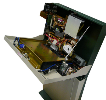
Computer components mounted on a hinged bracket for easy access
